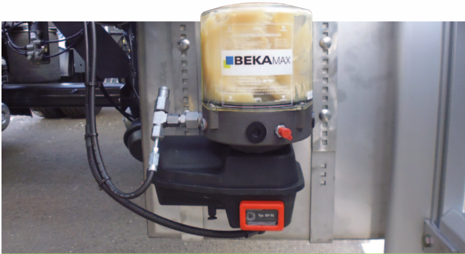
Automatic lubrication systems relieve the driver of regular lubrication of the relevant bearings.
