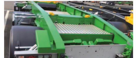
Aluminium chassis cover on the skid carrier
