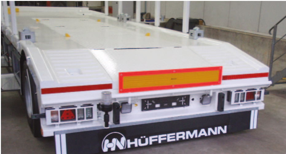
Trailer rear with protected tail lights, LED flashing lights in blue, work lights
